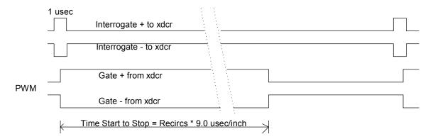
The tester issues one microsecond long interrogate+ and interrogate- pulses to the sensor. A good sensor will respond by changing the Gate + to high and the Gate – to low. The time from the leading edge of the PWM Gate+ signal until the trailing edge of the PWM Gate+ will be approximately 9 microseconds for each inch the magnet is from the head of the sensor times the number of recirculations programmed in the sensor. (9 \* magnet distance \* recirculations).
