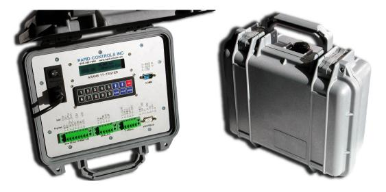
The Rapid Controls model TT Rev B transducer tester connects to multiple types of transducers and displays position and status information from the transducer. It is capable of testing SSI, PWM, Start/Stop, Neuter, Analog Output, CAN Open, MTS CAN bus and ProfiBus DP transducers. Transducer selection is accomplished via the front-panel keypad. The display is portable, housed in a plastic desktop enclosure, and optionally battery powered.
